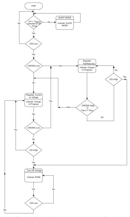
Figure 8. System-Controlled Operational Flow Chart
