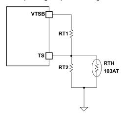
Figure 17. TS Resistor Network
