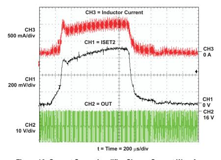
Figure 16. Current Sense Amplifier Charge Current Waveform
