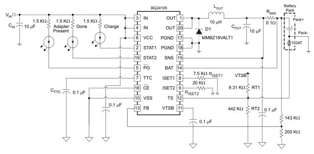
Figure 19. 1-Cell LiFePO4 Application
