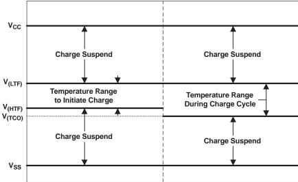
Figure 10. TS Pin Thresholds
