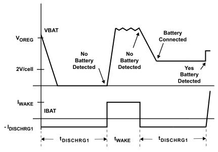
Figure 12. Battery Detect Timing Diagram
